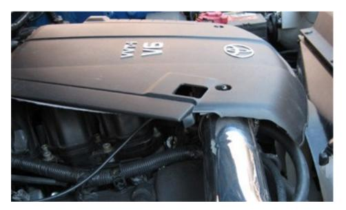
B. Install the plastic engine cover onto the rear mount and the driver's side mounting bolt. Note that some of the plastic will have to be
