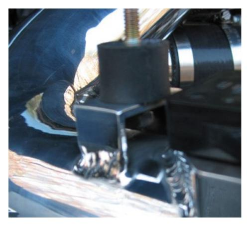
A. On the front section of intake piping, install the rubber lord mount into the mounting bracket. Tighten the nut with a 11mm wrench.
