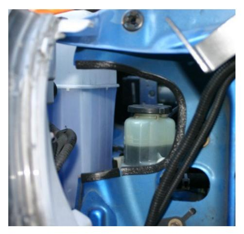
E. Place the included plastic combing material on the cut edge to prevent damage to components passing through the hole.
