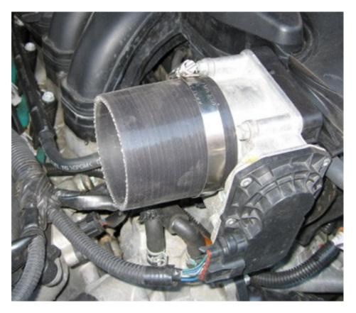
A. Install one of the silicone couplers on the throttle body. Slip two of the 3" liner clamps onto the coupler. Do not tighten.
