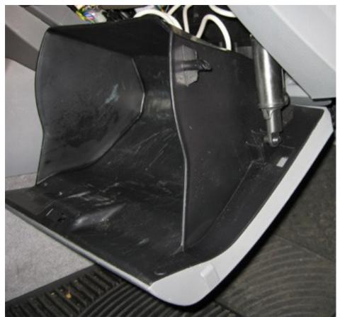
Note, the lower connection of the opening dampener should of already been removed and not still attached as in this picture.
