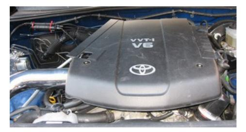
D. Reinstall the plastic engine cover and secure it with the stock acorn nuts.
