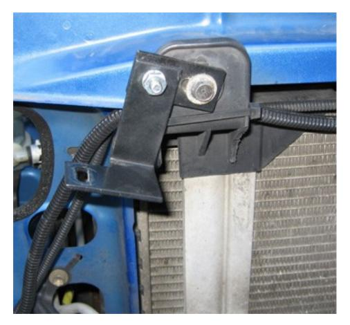
B. Remove the passenger side A/C condenser mounting bolt. Insert the support bracket as shown. Leave it loose for now.
