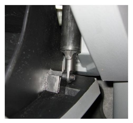
B. On the passenger side you will find an opening damper. Remove the lower attachment by squeezing the retaining barbs together. This will allow you to push the lower connection off of the mounting pin.
