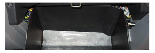
C. Push the sides of the glove box together enough to allow the opening limit stops on each side to pull past the sides of the dash.
