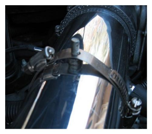
A. Loosely install the 3" clamp with the 6 mm bolt in it as shown. You will need to move it into final position later.
