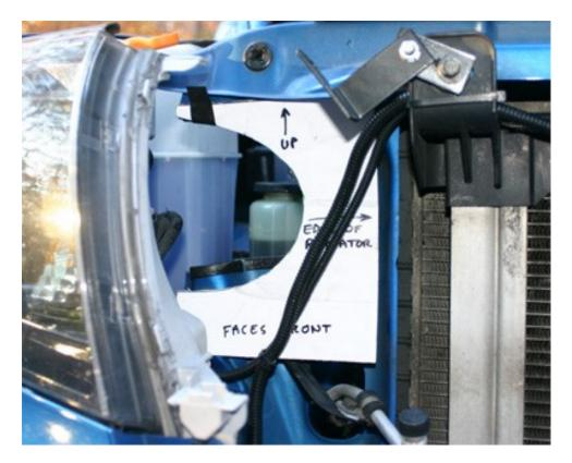
B. Place the template on the radiator support and trace the line to be cut with a Sharpie marker or grease pencil.
