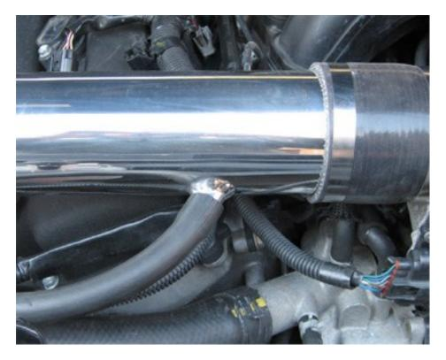
A. Connect the crankcase vent hose to the forward vent nipple on the main intake pipe as shown.
