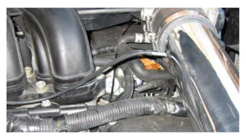
C. Connect the other end of the vacuum line to the smaller port on the rear side of the main intake tube.
